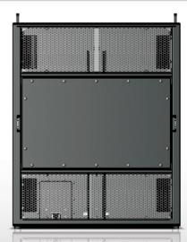
Subbass cabinet featuring a Neodymium high excursion 3000W 18" driver. A bandpass load ensures SPL output equivalent to conventional dual 18" subbasses. Same width, double the height of M46 main cabinet, double height of main cabinet so the S118 can be flown in the array or ground-stacked in line. Can be run in omnidirectional or cardioid sub mode.
