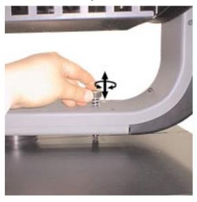
2) The second stop, located between the yoke and the lamp housing, inhibits the tilt movement of the lamp housing. Locate the stop and gently rotate it until it automatically releases itself
