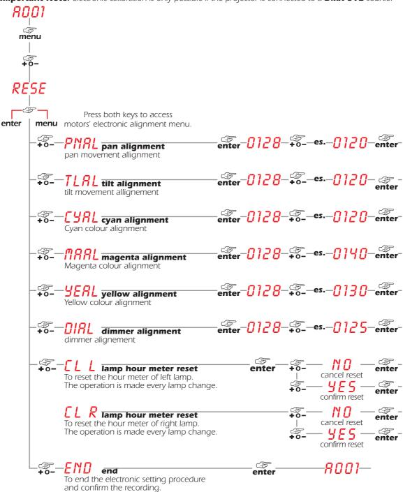
**Important Note:** At the termination of the above electronic calibration procedure, if the END function is not performed, no memory changes will be effected. This allows the operator to abort any changes made, in case of operator error.
