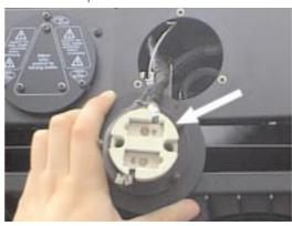
6) Insert the lamps. The lamps are manufactured from quartz glass and should be handled with care; always adhere to the instructions supplied in the lamp's packaging. Never touch the glass directly, use the tissue provided in the lamp's packaging. The G 22 lampbase is symmetrical. DO NOT USE UNDUE FORCE. In case of difficulty, inspect for physical damage and then repeat the installation procedure.
