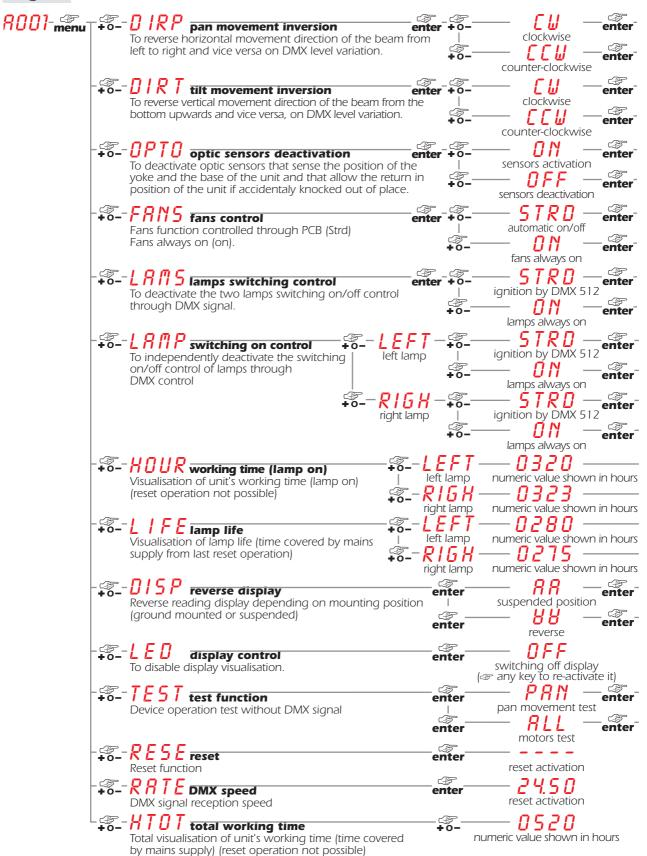
**12.1. Turning on the** *SuperCyc 2.4* without articulated movement
