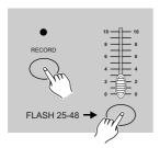
Press a Flash button between 25-48 while holding down the Record button. All LED will flash indicating the scenes have been programmed into memory.
