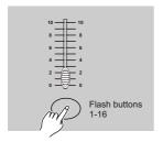
Tap the Flash button numbered from 1-16 to assign MIDI OUT channel 1-16, the relevant channel LED lights indicating MIDI OUT channel is set.
