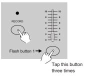
Tap the Flash button 1 three times while holding down the Record button, the Segment Display reads "CHI" indicating MIDI IN channel setup is available.
