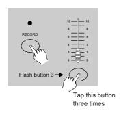
Tap the Flash button 3 three times while holding down the Record button, the Segment Display reads "IN" indicating the controller is ready to receive MIDI file dump.
