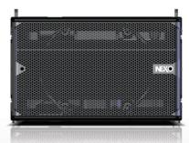
Injection-moulded bass cabinet featuring a Neodymium high excursion 3000W 12" bass driver with 4" voice coil. It has the same format – dimensions, weight, gravity centre – as the M46. The hybrid horn-loaded design maximizes the efficiency of the driver, delivering 6dB more than a standard front-loaded driver in this frequency range.
