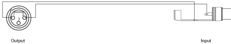
Cable to RCA input from balanced output. RCA and XLR connectors.
