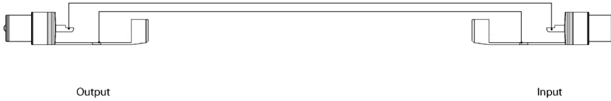
Cable to balanced input from balanced output. TRS and XLR connectors.
