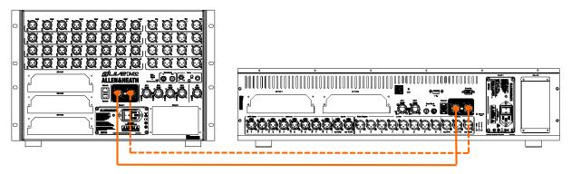
Switch on the Surface. The gigaACE Lnk/Err indicators flash at a steady rate when the link is established. The red error indicator lights if a communication error is detected. Check that the cables are correctly plugged in and are not faulty.
