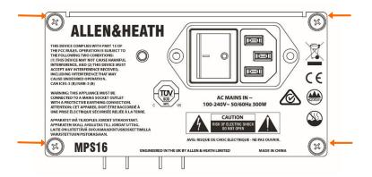
(i) dLive MixRacks ship with one PSU fitted. A second PSU can be fitted for redundancy (part number MPS-16). Loosen the 4 captive thumb screws securing the blank panel\*, slide the PSU into the slot, and tighten the 4 captive thumb screws indicated above. The MixRack will automatically switch between the supplies without interruption to the audio should one fail.
