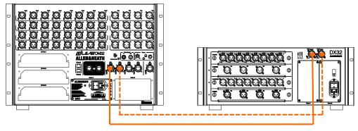
Switch on the DX Expander. The DX port Lnk/Err indicators flash at a steady rate when the link is established. The red error indicator lights if a communication error is detected. Check that the cables are correctly plugged in and are not faulty.
