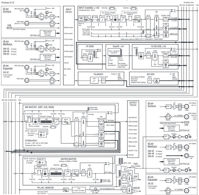
128 input channels x 64 bus Mix Engine
