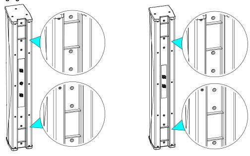
2 locations for connecting, 1 on the back and a quick connect in the base cover (ID84 only).
