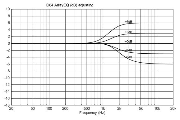
Apply the following array EQ HF on all ID84 (not ID84L) of the assembly:
