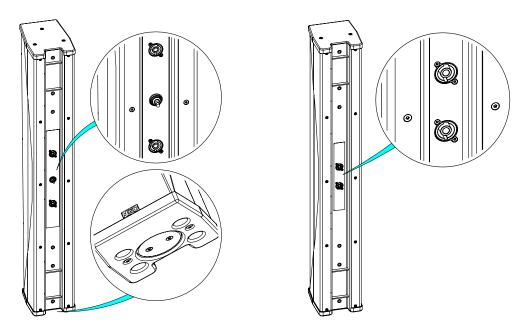
ID84 versions T & TIS: a directivity switch, located between the NL4 connectors, allows to virtually curve the drivers to achieve 2 vertical directivity patterns:
