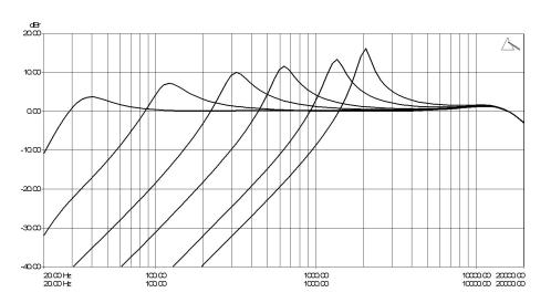
This graph illustrates how the resonance of the High-Pass Filter is automatically reduced as the frequency is lowered
