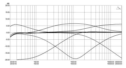
**BOOTH** - This section controls the level and frequency response of the Booth outputs. The Booth section incorporates a 2-Band equaliser allowing the user to adjust the frequency response of the Booth monitors to suit their own preference.
