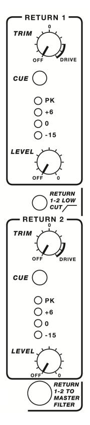
The Return section is located on the upper left-hand side of the front panel and consists of two basic stereo channels for use as return inputs from external effects processors. Connection to the Return channels is via  $4 \times 1/4^{"}$  TRS Jack sockets mounted on the rear panel, however the Return channels can also be fed from the DB25 connector DSUB IN 2 - see page 12 for details.
