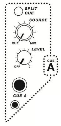
**MODEL 1** has two independent Cue systems, A and B. Cue A routes to the right hand side headphone monitor and the Cue B routes to the left hand headphone monitor. The dual Cue system makes it much easier for two DJs to perform on the mixer together as each can select a separate channel to monitor without interfering with the other performer's monitoring. This dual system also allows for Cue interaction between two mixers linked together. See page 13 for details of mixer linking.
