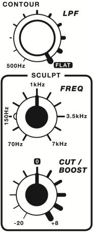
**MODEL 1** provides a unique alternative to the standard type of fixed frequency EQ, which we feel offers greater creativity and the ability to perform smoother mixes. Whereas a standard EQ has three or four controls providing cut or boost at a fixed frequency, **MODEL 1** utilises a combination of high and low pass filters plus a wide frequency range, swept equaliser, with asymmetric cut and boost.
