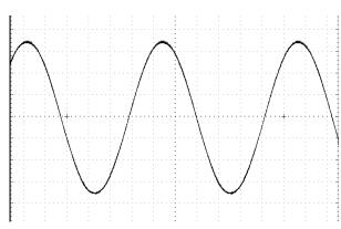
This trace shows two signals, one running through the drive circuit and one not. As the clip threshold has not been reached, both signals are identical.
