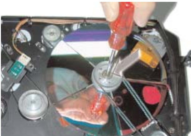
Figure W15C: Loosening Color Wheel Screws
