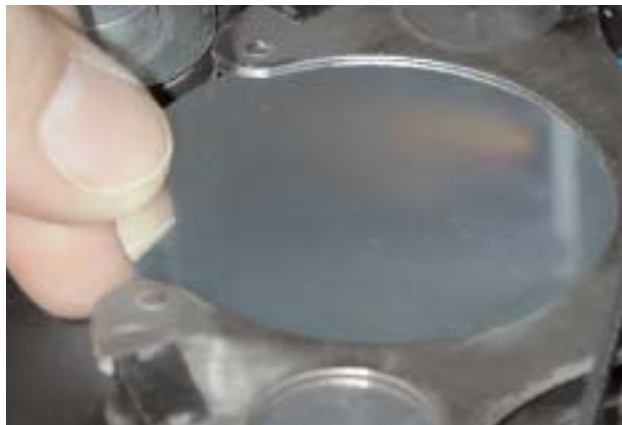
Figure W16 Removing Color Filter
