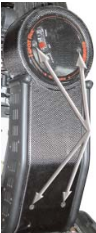
Figure W13A Removing Yoke Covers
