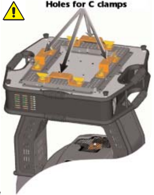
Figure W5 showing clamps fitted
