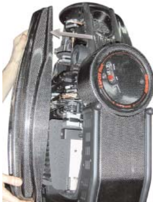
Figure W12B Removing Fixture Covers
