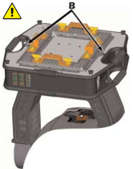
Figure W6 showing safety cables fitted
