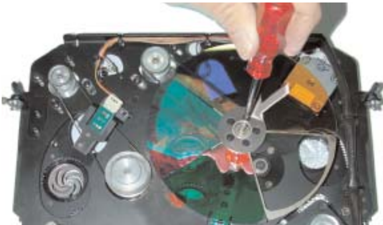
Figure W15B: Loosen Screws on Color Wheel
