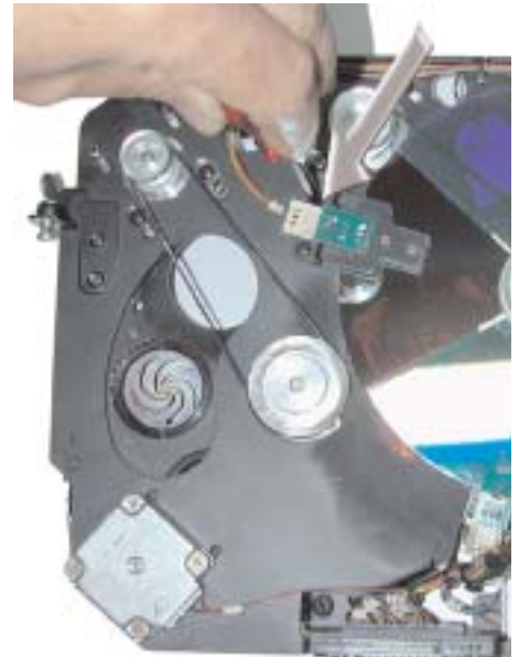
Figure W15A: Removing Sensor
