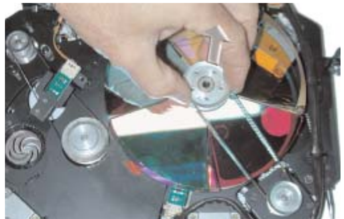
Figure W15D: Removing Color Wedges
