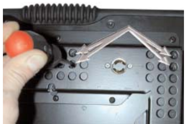
Figure W11B - Removing Switching Supply
