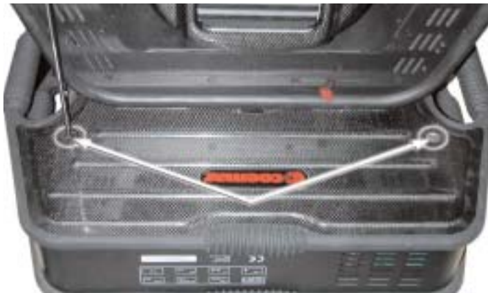
Figure W11A - Removing Base Covers
