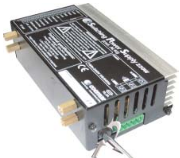
Figure W11D - Changing Switching Supply Fuse
